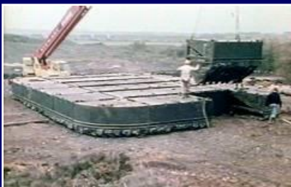
Modular Hoverbarge 1974 Length 24.34 m Width 13.4m All up Weight 110t Payload 50t
