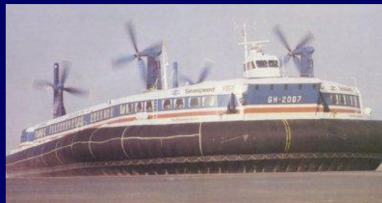
SRN4 1968 (Mk 1) Length 39.68m Width 23.77m All up Weight 167.8t Payload 64.5t
