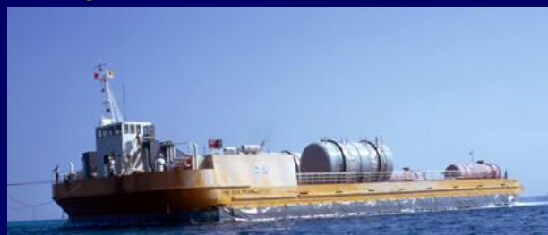
Sea Pearl 1976 Length 55m Width 24m All up Weight 750t Payload 250t
