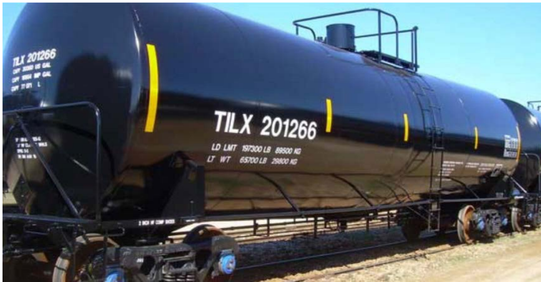
Figure 22 Insulated Tank Car with Coil Heating
