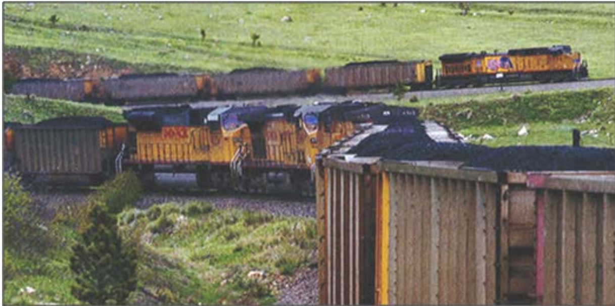
Figure 6 Photo of Distributed Power in use within a Single Coal Train
