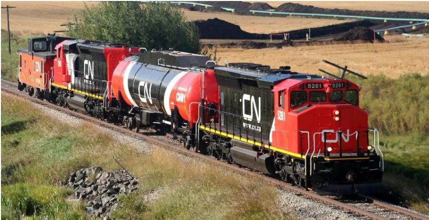
Figure 24 LNG Locomotive with Tender Car tested by Canadian National Railway
